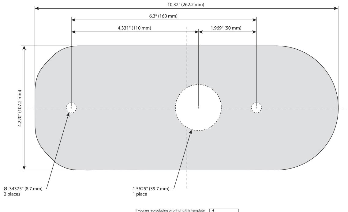
from an electronic file, adjust the enlargement or reproduction value in the page setup window to 100%. Measure the reference square (25.4 mm x 25.4 mm with a ruler and adjust your reproduction setting (%) to produce a print so that the square measures 1" x 1" or 25.4 mm x 25.4 mm.
