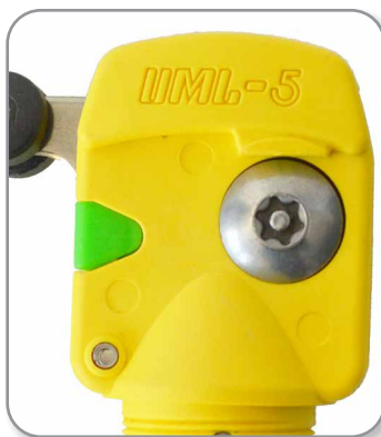
Uses a TX30 Torx Bolt A Torx adaper will be required to tighten the unit to 3nm
